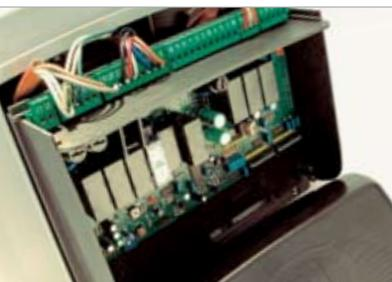
**A safe system.** In all of the versions, the control electronics are built-into the unit (except for version BK2200T) and is protected from environmental agents.
